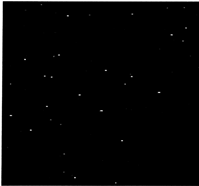
Fig. 4. Unrecoverable specks of CCD image sensor (DT neutron fluence: 8 \times 10^7 n/cm 2 , CCD sample: IC \times 054).
